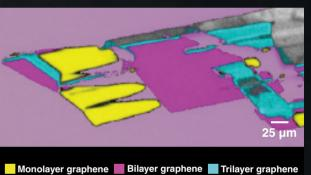
Raman image of varying thicknesses of graphene overlaid on a high-magnification optical image.
