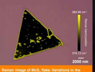
Raman image of MoS<sub>2</sub> flake, variations in the Raman band position were used to detect defects down to 250 nm.
