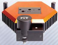
The Flex AFM Atomic Force Microscope from Nanosurf can be used to characterize the surface topography of battery materials and components. The AFM tip can also be made electrically active and used as a probe for nanoscale conductive/ resistive pathways. Measurements can be done within an electrochemical cell to passively observe changes due to charge/discharge events.
