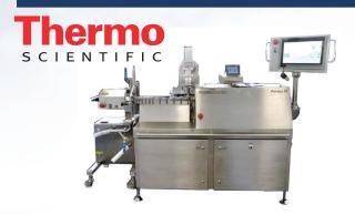
Thermo Scientific helps innovate in dry or low-solvent electrode manufacturing. The twin-screw extruder compounds anode material with minimized solvent addition. The highly viscous pastes are processed into pellets which are easily transported and stored without aging. The pellets can later be coated onto collector foil and calendared in one step.
