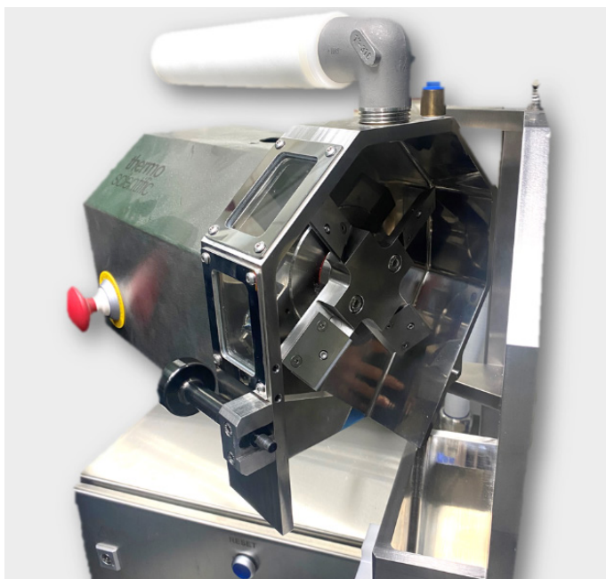
Figure 2: Pharma FaceCut 16 pelletizer cuts extruded paste into pellets with rotating blades directly at the die exit.
