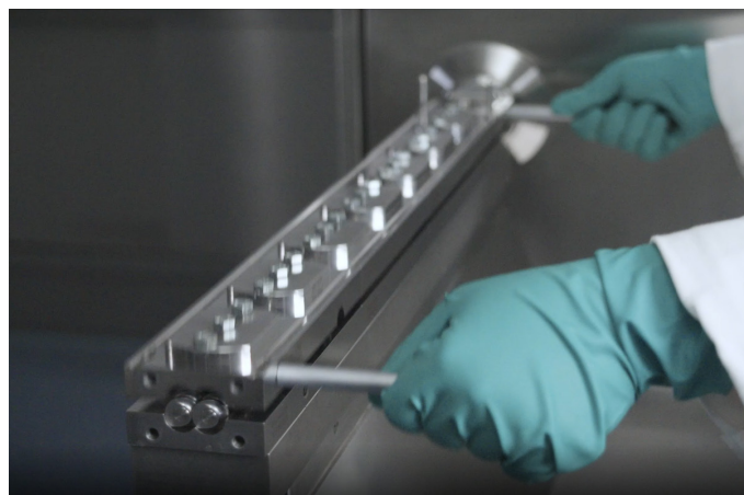
Figure 3: Split barrel design of Thermo Scientific Twin-Screw Extruder.
