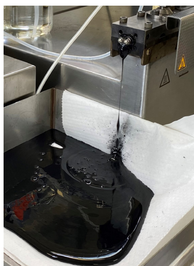
Figure 1: Thermo Scientific Cathode slurry compounded using Process 11 Twin-screw Compounder.
