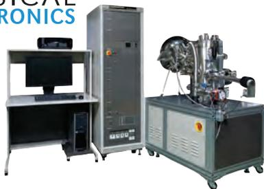
**X-ray Photoelectron Spectroscopy (XPS)** from **Physical Electronics (PHI)** is an important tool for battery material research and development. XPS can provide insights into battery performance at realistic operating conditions, and help determine the precise location of interfaces between battery components. Electronic band structure of organic and inorganic materials can also be characterized using XPS.
