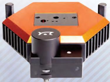
The Flex AFM Atomic Force Microscope from Nanosurf can be used to characterize the surface topography of battery materials and components. The AFM tip can also be made electrically active and used as a probe for nanoscale conductive/ resistive pathways. Measurements can be done within an electrochemical cell to passively observe changes due to charge/discharge events.
