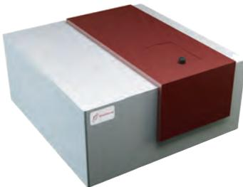
Battery particle charge (zeta potential) can affect slurry production and stability. The **Brookhaven Instruments NanoBrook Omni** provides fast, routine measurement of submicron particle size and zeta potential. This technology will help you understand sedimentation and agglomeration.
