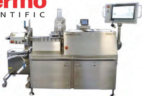
**Thermo Scientific** helps innovate in dry or low-solvent electrode manufacturing. The twin-screw extruder compounds anode material with minimized solvent addition. The highly viscous pastes are processed into pellets which are easily transported and stored without aging. The pellets can later be coated onto collector foil and calendared in one step.
