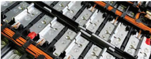
Lithium-ion batteries are the main energy storage technology for mobile devices such as smartphones and laptops. The wettability of different parts of Li-ion batteries has become one of the key issues both in terms of manufacturing as well as for the performance and safety of batteries.
