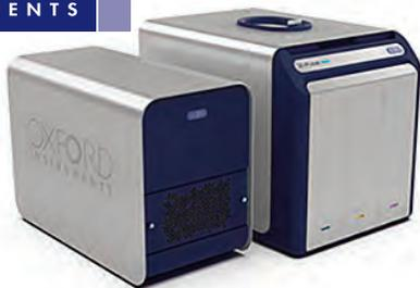
Electrolytes are a key component in battery performance. **Oxford Instruments'** benchtop NMR technology can quickly and easily distinguish between the diffusion behavior of different electrolyte solvents and help characterize important parameters such as conductivity and ion transference. For battery R&D, the Oxford Instruments **X-Pulse Broadband Benchtop NMR Spectrometer** provides critical data for electrolyte design.
