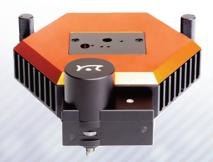
The Flex AFM Atomic Force Microscope from Nanosurf can be used to characterize the surface topography of battery materials and components. The AFM tip can also be made electrically active and used as a probe for nanoscale conductive/resistive pathways. Measurements can be done within an electrochemical cell to passively observe changes due to charge/discharge events. Learn more, download Nanosurf Flex AFM.
