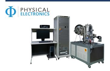
X-ray Photoelectron Spectroscopy (XPS) from Physical Electronics (PHI) is an important tool for battery material research and development. XPS can provide insights into battery performance at realistic operating conditions, and help determine the precise location of interfaces between battery components, electronic band structure of organic and inorganic materials, and other properties crucial to battery performance. Learn more, download the PHI XPS app.
