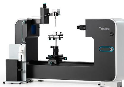
Theta Pulsating Drop can be based on the optical tensiometers Theta Flex or Theta Flow. The system supports measurements of interfacial rheology with the pulsating drop method.
