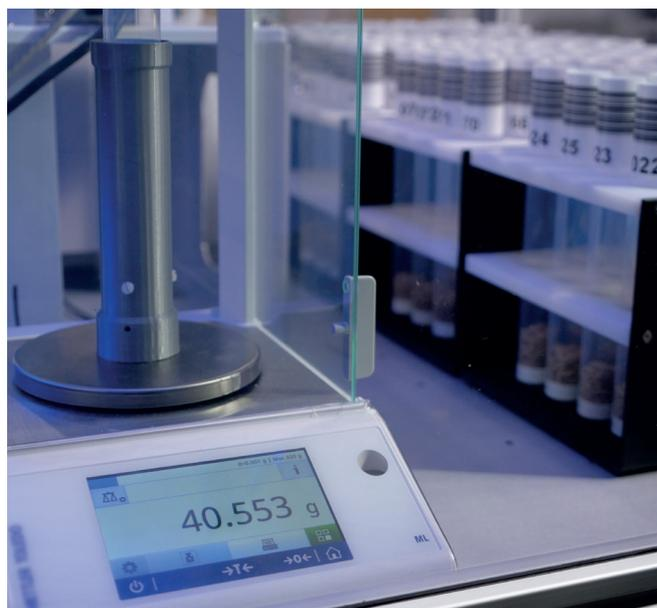
The optional balance automatically records gross weight of sample plus tube.
