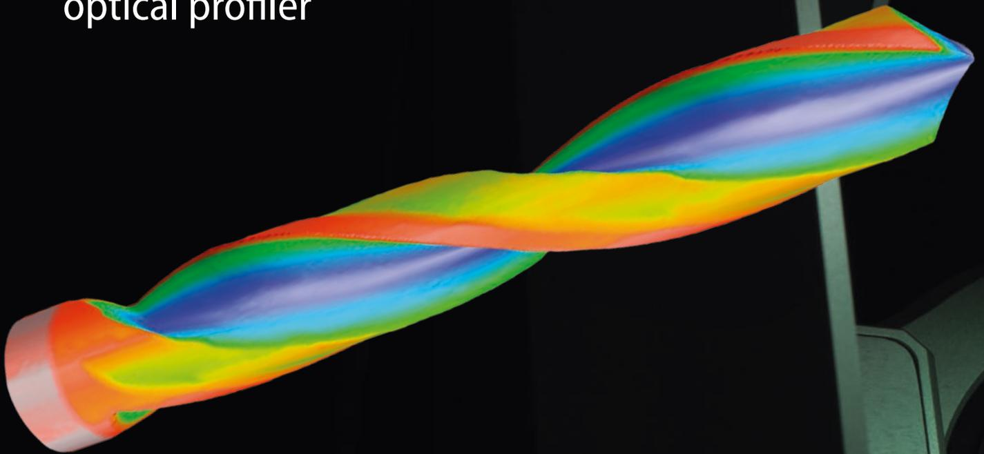
This enables automatic 3D surface measurements at defined positions which can be combined to create a complete 3D volumetric measurement. S neox 3D measurement technologies cover a wide range of scales, including form (Ai Focus Variation), sub nanometric roughness (Interferometry) or critical dimensions that require high lateral resolution as well as vertical resolution (Confocal).
