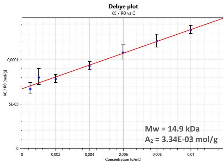
Figure 8: “Corrected” Debye plot of Lysozyme in 0.1M KCl in the case only the intensity scattered by monomers is processed. The values of  $KC/R(\theta)$  are plotted as a function of sample concentration (blue dots). The red line show the corresponding linear regression.
