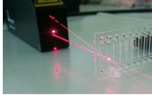
Figure 2: in-situ optical head of "VASCO Kin".
