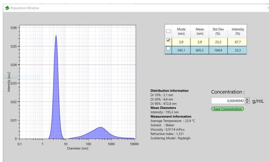
Figure 7: “NanoKin” software panel showing the DLS sizes measurement of Lysozyme in 0.1M KCl buffer at 0,000499g/mL. This window also allows to select on which population is processed the Mw calculation.
