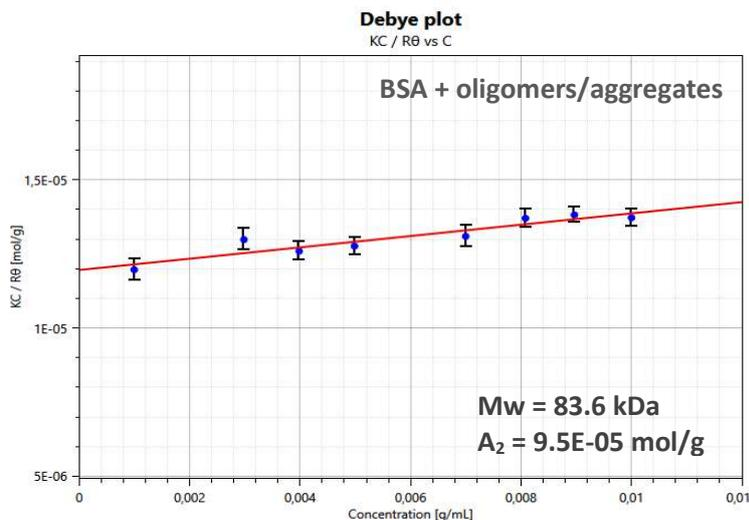
Figure 5: “Raw” Debye plot of BSA in 0.1M KCl in the case the whole sample scattering intensity is processed. The values of  $KC/R(\theta)$  are plotted as a function of sample concentration (blue dots). The red line show the corresponding linear regression.
