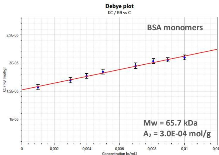
Figure 6: “Corrected” Debye plot of BSA in 0.1M KCl in the case only the intensity scattered by monomers is processed. The values of  $KC/R(\theta)$  are plotted as a function of sample concentration (blue dots). The red line show the corresponding linear regression.
