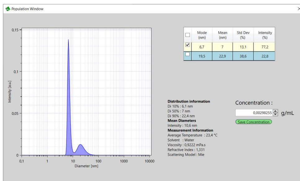
Figure 4: "NanoKin" software panel showing the DLS sizes measurement of BSA in 0.1M KCl buffer at 0,00298g/mL. This window also allows to select on which population is processed the Mw calculation.
