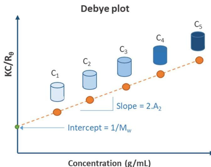
Figure 3: Debye plot. Values of  $KC/R(\theta)$  are plotted as a function of sample concentration. The slope of the corresponding linear regression is equal to  $2x A_2$  while the intercept at  $C=0$  is equal to  $1/M_w$ .
