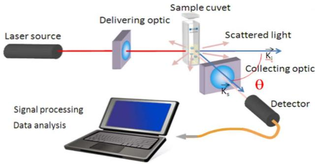
Figure 1: General set up of a light scattering experiment.
