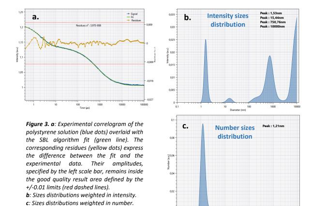
The size distribution in intensity (figure 3.b) shows that several populations are detected in the sample. In particular, we clearly observe a population having a hydrodynamic diameter of **1.53nm** (peak mode), consistent with the expected size range for such polystyrene coils in toluene.
