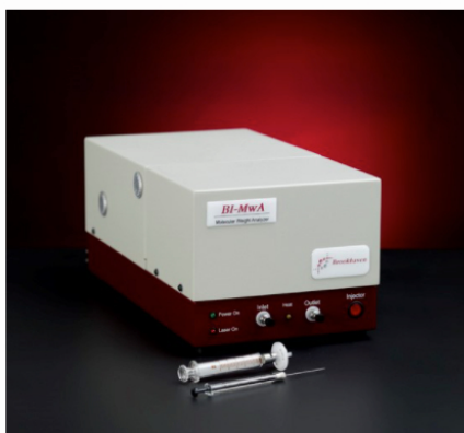
The BI-Molecular Weight Analyzer, a Multi-Angle Static Light Scattering System
