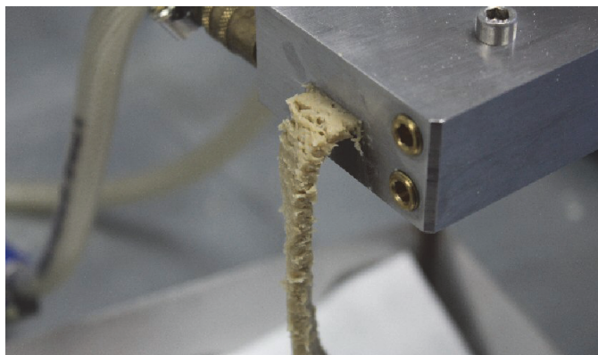
Special die for the extrusion of plant-based proteins samples.
