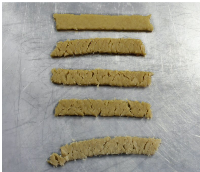
Wheat gluten samples with different textures. From top to bottom: The samples develop the fibrous characteristic of meat by optimizing the extrusion conditions.
