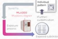
The benefit of Maskless Lithography is the inherent rapid turnaround and adaptation of the exposed patterns. Adaptations for customized products or even simply a large product portfolio no longer entail the time and cost of production and maintenance of an expensive mask set. Switching between product types is seamless, and does not require intervention to change masks.
