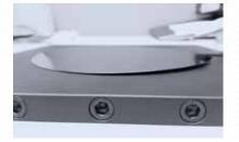
Structuring flexible substrates is challenging as the shape and the distortions vary with applied forces. Maskless lithography offers the unique option of exposing the substrates with warpage-dependent pre-distortions, to maximise yield
