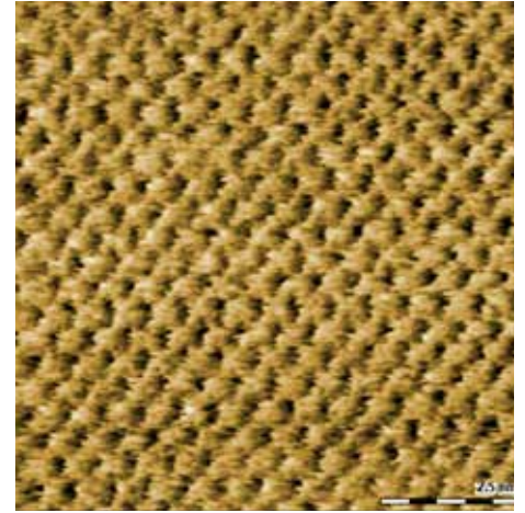
Atomic grid on mica measured with lateral force microscopy
