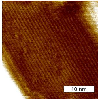
**Lamellae in polyethylene**
