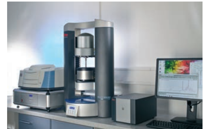
Modular rheometer platform HAAKE MARS with Rheonaut module and Thermo Scientific™ Nicolet™ iS™10 FT-IR spectrometer
