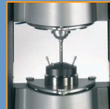
Temperature module for parallel plates with sample hood
