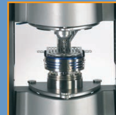
Electrical temperature module for parallel plates with active upper heater
