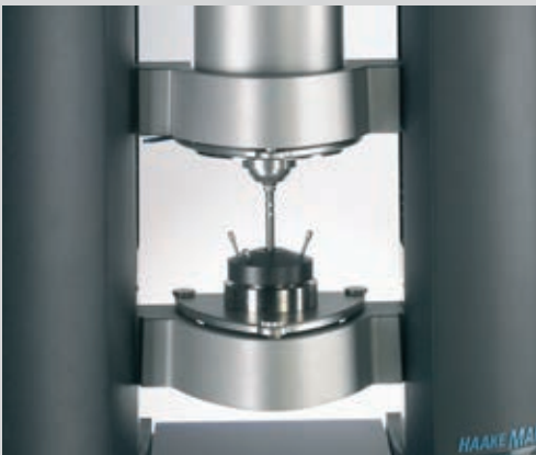
HAAKE MARS with Peltier Temperature Module, parallel plates and sample hood with solvent trap
