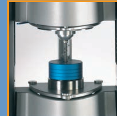
Temperature module for parallel plates with Insulated sample hood
