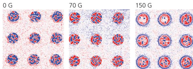
**Figure 6: Magnetic skyrmions in Co-based thin film pads**
