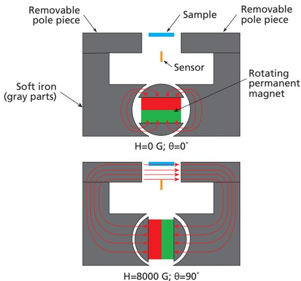
**Figure 2: Schematic of in-plane field configuration**
