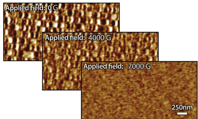
**Figure 3: Degaussing bits on PMR hard drive**
