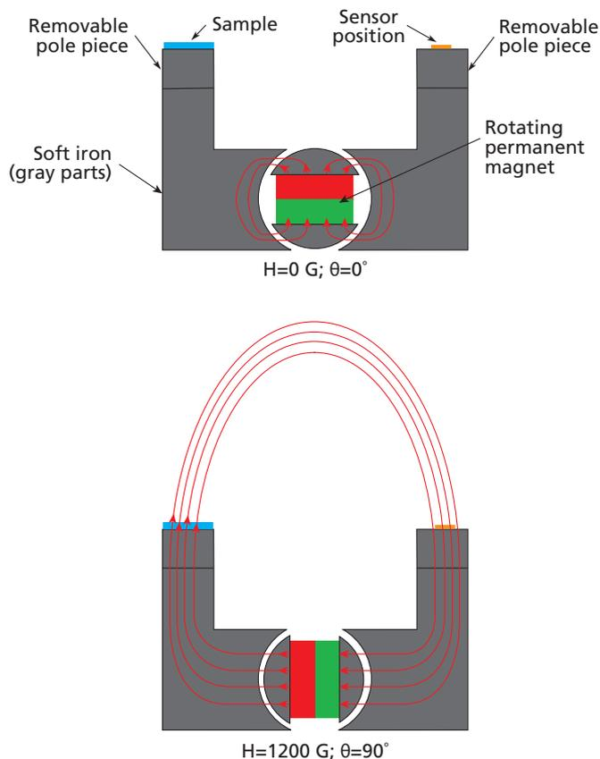
**Figure 5: Schematic of out-of-plane field configuration**
