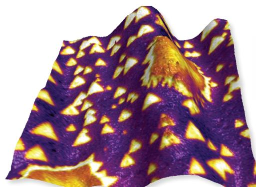
**Boron nitride and graphene grown on copper film** imaged using KPFM. Surface potential data is shown on 3D topography, clearly showing triangular patches of boron nitride and irregular areas of graphene that would have otherwise been obscured by the rough topography of the copper, 50  $\mu\text{m}$  scan. Sample courtesy of N. Wilson, University of Warwick.
