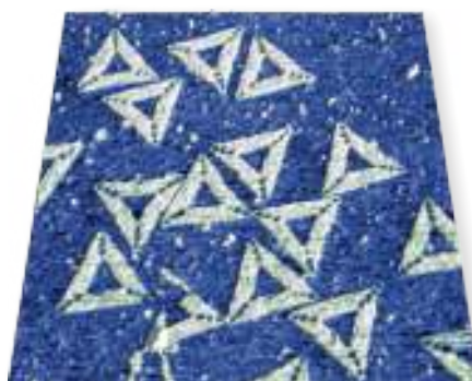
DNA origami triangles , imaged in fluid, 600 nm scan. Sample courtesy of P. Rothmund, California Institute of Technology.
