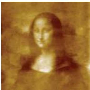
Nanolithography example created by anodic oxidation on silicon, 20 \mu\text{m} scan.
