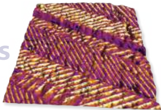
Molecular ferroelectric film PFM phase data is shown on 3D topography, 20 \mu\text{m} scan. Image courtesy of A. Eshghinejad and J. Li, University of Washington.
