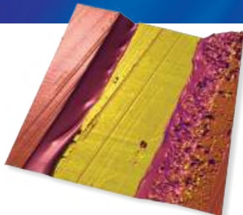
Multi-layered coffee bag cross-section imaged using AM-FM Viscoelastic Mapping Mode. Modulus data is shown in 3D topography, 30 \mu\text{m} scan.
