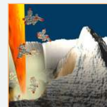
Illustration of the NanoFrazor creating a nanoscale Matterhorn [1]
