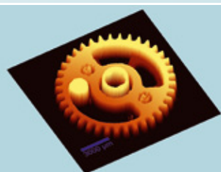
2.1 Large area topography profilometer measurement of a micromechanical gear (15 x 15 mm).
