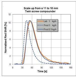
Fig. 6: Residencwe time for scale up tests
