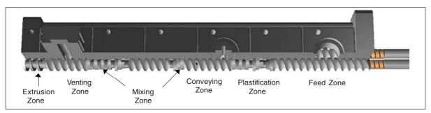
Fig. 1: Barrel and screw layout
