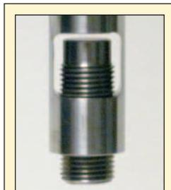
Figure 2: Transfectance probe used in the analysis, showing detail of adjustable pathlength.
