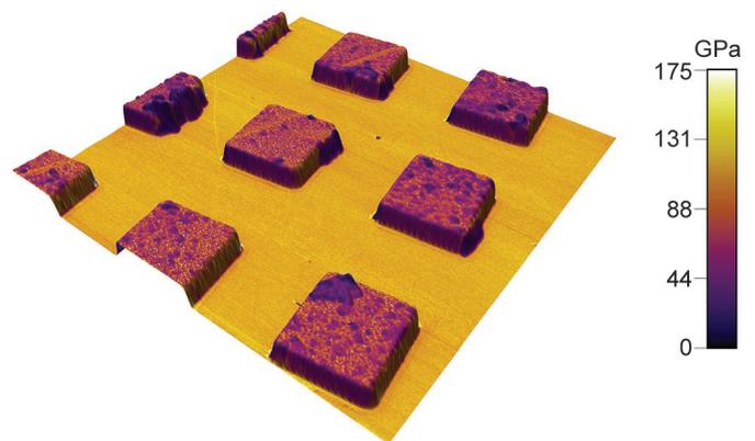
**Figure 10:** Elastic modulus image of a patterned titanium film on silicon, overlaid on topography. blueDrive photothermal excitation on the Cypher AFM was used for DART contact resonance imaging. Note the strong contrast between these two very high modulus materials. Scan size 25  $\mu\text{m}$ .
