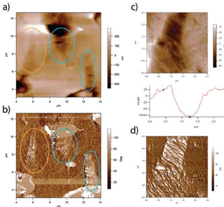
Figure 5: Corresponding topography (a) and phase (b) images of  $15\mu\text{m} \times 15\mu\text{m}$  area of PP matrix within ICP material at 2% elongation. Regions of large crack formation are highlighted in orange and blue circles. Zoom in on crack highlighted in orange circle in (a) is shown in corresponding topography (c) and phase (d) images. Line scan in (c) along red line measures width and depth of crack.
