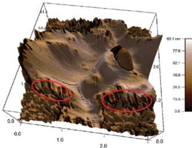
Figure 4: 2nd mode amplitude overlaid onto 3-D topography of ICP material rendered from Figure 3b. Interface showing stretching of the EP domain as it adheres to the PP is circled in red.
