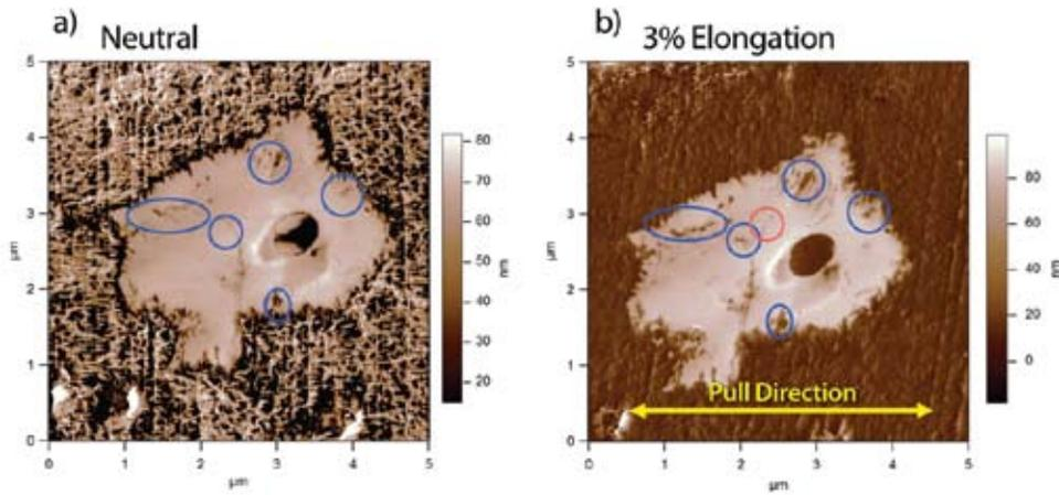
Figure 2: Amplitude mode 2 images of identical EP domain within ICP material at (a) neutral position on NanoRack and (b) 3% elongation on NanoRack.
