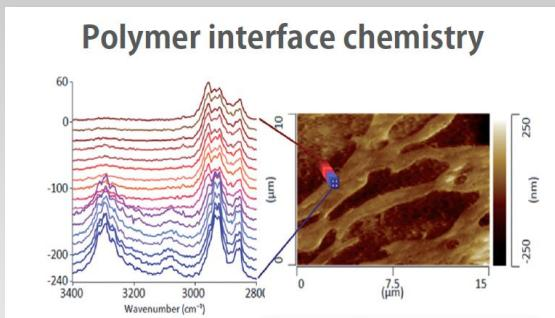
Direct IR absorption spectroscopy & chemical imaging
